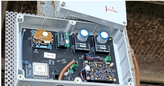
Control unit for monitoring the quality of the environment (gas concentrations, noise)
