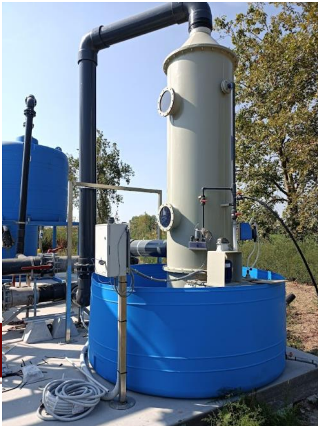
The scrubber cleans the ammonia-charged air exiting the reactors to form ammonium sulphate which can be used as a fertilizer
